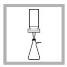
4. Invert the sample for 30 seconds to mix. Pour 100 mL of sample into the funnel. Apply vacuum and filter the sample. Release the vacuum. Rinse the funnel walls with 20 to 30 mL of sterile buffered dilution water. Apply vacuum. Repeat rinsing step 2 more times.
