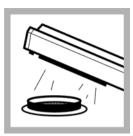
7. Using a long-wave UV lamp, examine the colonies for fluorescence. Fluorescence indicates the presence of *E. coli.*
