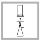
5. Turn off the vacuum and lift off the funnel top. Using sterilized forceps, transfer the filter immediately to the previously prepared petri dish.
