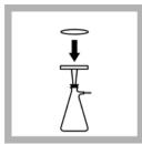
3. Set up the Membrane Filter Assembly. Use sterilized forceps to place a membrane filter, grid side up, into the assembly. Alternatively, a sterile disposable filter unit may be used.
